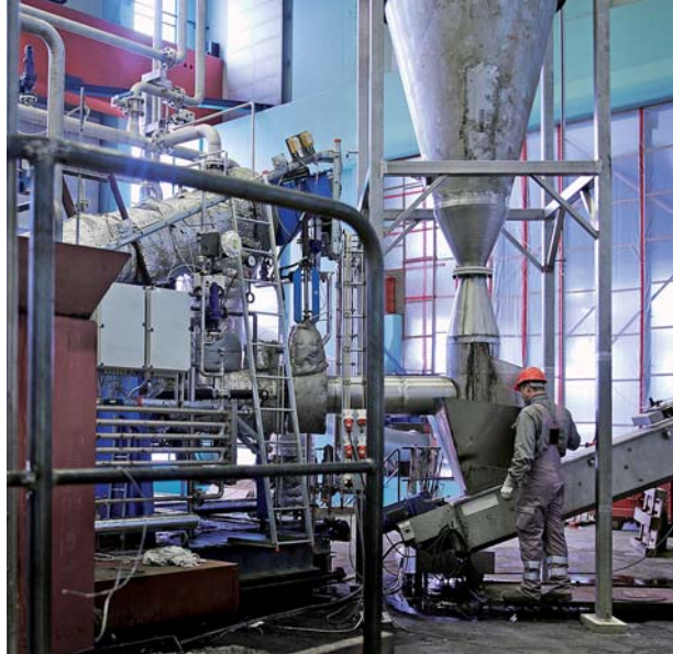
C5/C6 sugar and lignin platform biorefinery for ethanol, animal feed, power and heat from lignocellulosic residues. Courtesy Inbicon IBUS, Denmark; and Task 42.
