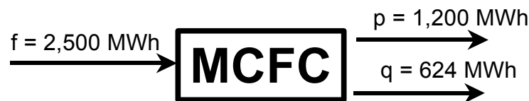
Figure 22 — MCFC Energy Balance
