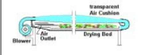
Figure 5: Examples of solar Dryers: Stacked grids (left) and horizontal bed dryer with air- filled cushion (below)
