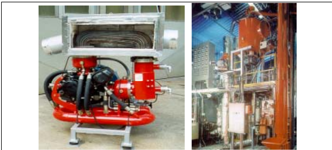
Fig. 6: 3 kW Stirling engine for biofuel operation at JOANNEUM RESEARCH, Austria (left); flash pyrolysis plant at VTT, Finland (right)
