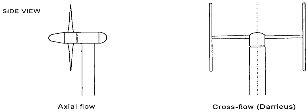
Fig. 5. Schematic representation of the axial-flow and cross-flow rotors.
