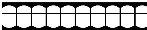
Figure 6 Principle of the cross-section of the polymer absorber. Water fills the upper, smaller channels.
